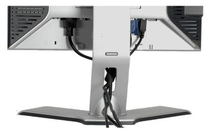
After attaching all necessary cables to your monitor and computer, (See <u>Connecting Your Monitor</u> for cable attachment,) use the cable holder to neatly organize all cables as shown above.
