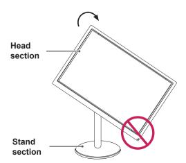
3 Be careful with the cables when rotating the screen.
