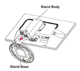
3 Using a coin, turn the screw clockwise to secure the stand base.
