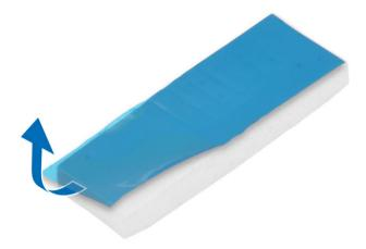
4 Place the rubber on the system board [1] and peel the adhesive tape (pink) from the rubber [2].
