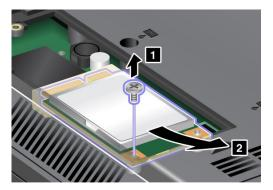
6. Align the contact edge of the new mSATA solid state drive with the corresponding socket and pivot the mSATA solid state drive until you can snap it into place. Secure the mSATA solid state drive with the screw.
