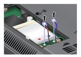
6. Remove the screws and the card pops up. Remove the card.
