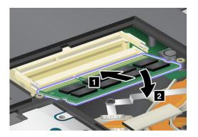
Note: Insert the SO-DIMM into the socket at an angle of about 20 degrees.
