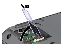
7. Insert the SIM card firmly into the card holder and pivot the card holder downward.
