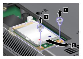
7. Align the contact edge of the new PCI Express Mini Card with the corresponding socket. Pivot the card until you can snap it into place. Secure the card with the two screws.
