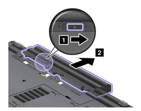
5. Insert a fully charged battery until it clicks into place 1 as shown in the drawing, and then slide the battery latch to the locked position 2.
