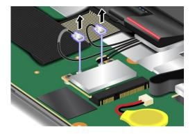
7. Remove the screws and the card pops up. Remove the card.
