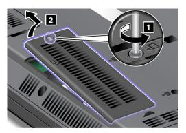
5. Remove the screw and the mSATA solid state drive pops up. Remove the mSATA solid state drive.
