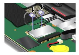
Note: Be sure to attach the gray cable to the connector marked "MAIN" on the card and the black cable to the connector marked "AUX".
