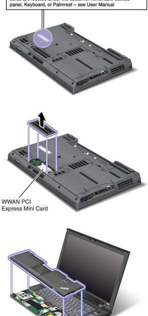
If no integrated wireless PCI Express Mini Card has been preinstalled in your computer, you can install one. To do this, follow the procedure in "Replacing the PCI Express Mini Card for wireless LAN/WiMAX connection" on page 110 or "Installing and replacing the PCI Express Mini Card for wireless WAN connection" on page 111.
