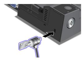
Attach a mechanical lock to the ThinkPad Port Replicator Series 3 as follows:
