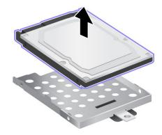
9. Place the new drive into the bracket as shown in the drawing.
