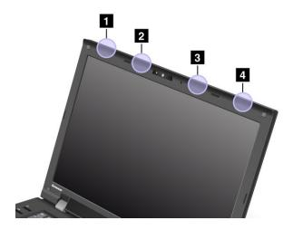
1 Wireless LAN and WiMAX combo antenna (Auxiliary)
