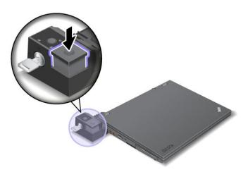
3. Press the eject button 1 until the computer moves up, then, grasping both sides, remove the computer
