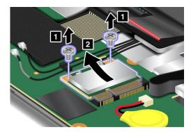
8. Align the contact edge of the new card with the corresponding socket contact of the computer. Pivot the card until you can snap it into place and secure the card with the two screws.
