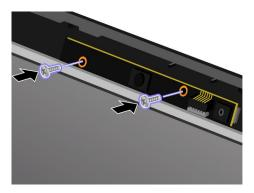
8. Reinstall the LCD bezel assembly.
