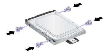
11. Turn the hard disk drive over again and place the hard disk drive from the right side as shown in the picture.
