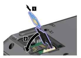
8. To lock the card holder, slide it as shown in the drawing.
