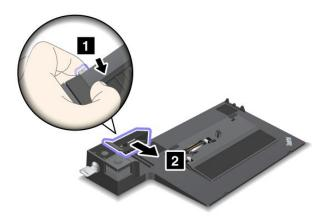
3. Put your computer on the platform of the ThinkPad Mini Dock Series 3, or the ThinkPad Mini Dock Plus Series 3, making sure that the top-left corner of the computer is aligned to the guide plate on the ThinkPad Mini Dock Series 3, or the ThinkPad Mini Dock Plus Series 3.
