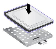
10. Reinstall the screws to secure the bracket.
