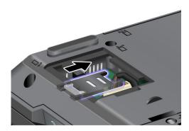
6. Lift up the card holder and then remove the dummy card. Keep the dummy card for future use.
