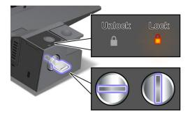
When the key is in the locked position, the eject button of the ThinkPad Mini Dock Series 3, or the ThinkPad Mini Dock Plus Series 3 is locked, and you cannot remove your computer. The key lock indicator lights when the eject button is locked.
