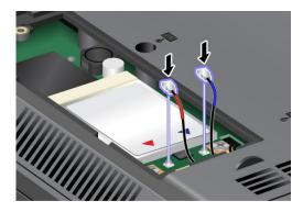
Note: Be sure to attach the red cable to the Main connector, and the blue cable to the AUX connector.
