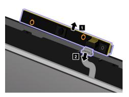
6. To install a new camera, attach the connector 1 and position the camera in place 2.
