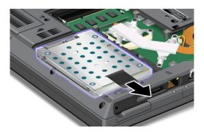
6. Remove the hard disk drive by lifting its left side.
