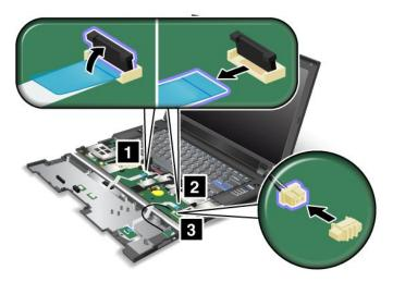
8. Release the palm rest from the computer. Now the palm rest has been removed.
