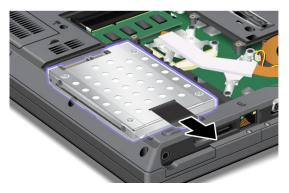
6. Remove the solid state drive by lifting its left side.
