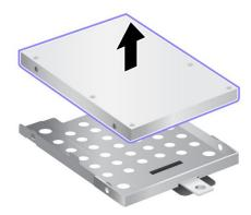
9. Place the new drive into the bracket as shown in the drawing.
