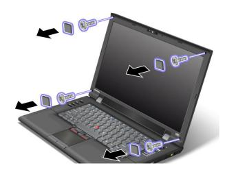
3. Remove the LCD bezel assembly.
