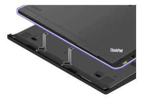
2. Ensure that the guides of the ThinkPad Battery 19+ align with the holes in the computer 1. Then secure the computer in place 2.
