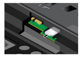
5. Insert the new SIM card firmly into the slot.
