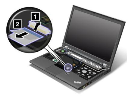
7. Lift the palm rest up and remove it.
