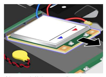
9. Align the contact edge of the new card with the corresponding socket.
