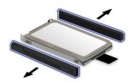
7. Attach the side rubber rails to the new hard disk drive or the side spacer rails to the new solid-state drive.
