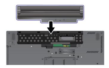
6. Make sure that the battery latch to the locked position.
