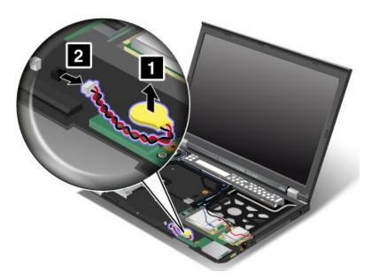
7. Put the new backup battery in place and connect the cable.
