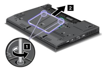
If two memory modules already are installed in the memory slots, remove a memory module to make room for the new one by pressing out on the latches on both edges of the socket at the same time 1 and removing the memory module 2. Save the removed memory module for future use.
