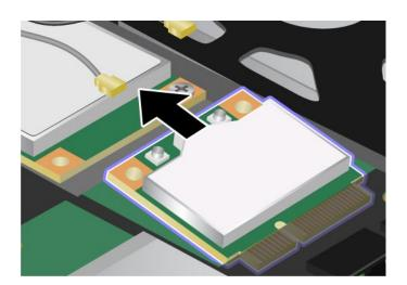
9. Align the contact edge of the new card with the corresponding socket.
