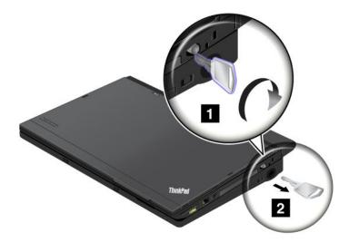
Note: You can turn the key clockwise to lock it. Then, keep the key in a safe place. Do not lose this key; otherwise, you will be unable to detach the computer from the ThinkPad UltraBase Series 3.
