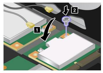
11. Connect the cables to the new wireless LAN/WiMAX card. Ensure that you attach the gray cable to the connector marked TR1 or Main on the card, and the black cable to the connector marked TR2 or Aux.
