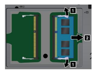
5. Find the notch on the contact edge side of the memory module you are installing.
