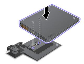
4. Insert your computer into the docking station until you hear a click. The computer is attached to the docking station.
