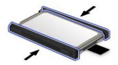
8. Insert the new hard disk drive or solid-state drive into the slot.
