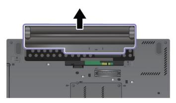
5. Slide the new battery into the computer.
