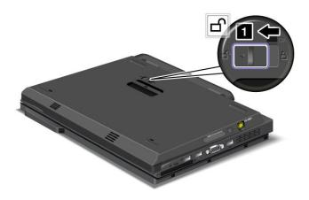
2. Release the eject lever 2 and detach the ThinkPad Battery 19+.
