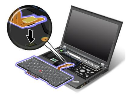
2. Insert the keyboard. Make sure that the rear edges of the keyboard are under the frame.
