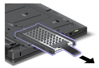
6. Detach the side rubber rails from the hard disk drive or the side spacer rails from the solid-state drive.
