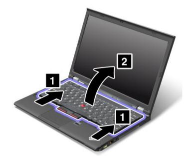
7. Carefully lift the keyboard until you can see how it is connected. Hold the keyboard above the computer **1**, and then detach the connector **2**. Remove the keyboard.
