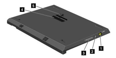
1 Power jack: The is where you connect the ac power adapter.
