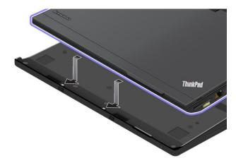
3. Ensure that the guides of the ThinkPad UltraBase Series 3 align with the holes in the computer 1. Then secure the computer in place 2. The docking status indicator lights.
