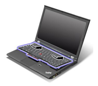
3. Press gently on the keyboard and slide the keyboard in the direction shown by the arrows. Make sure that the edges of the keyboard are under the frame.
