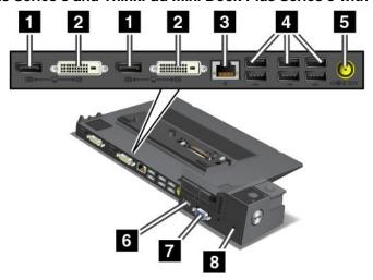
1 3 DisplayPort connector: Connect a display device.
