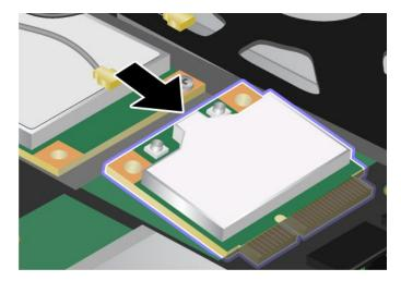
10. Pivot the card until you can snap it into place by pressing the upper side of the connectors, and secure the card with the screw.
