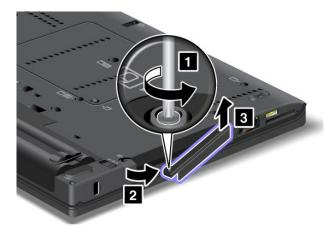
5. Remove the hard disk drive or solid-state drive by pulling out the tab.
