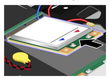
10. Pivot the card until you can snap it into place by pressing the upper side of the connectors, and secure the card with the screw.
